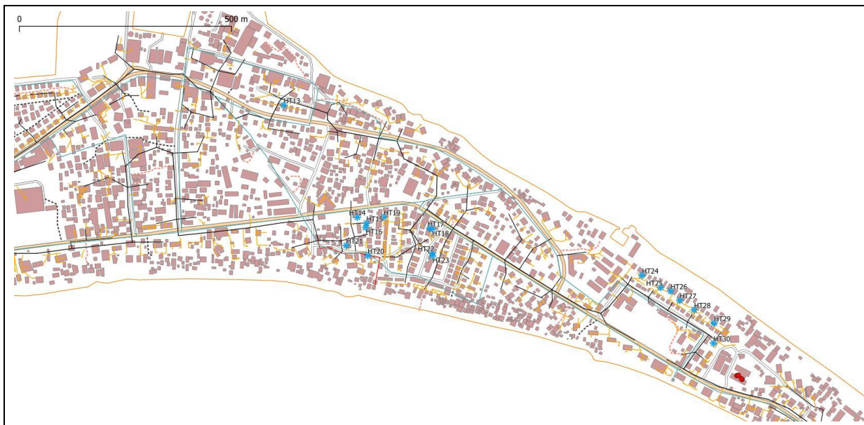
Figure 4: KHC communal toilets in East Betio relative to the main sewer line
